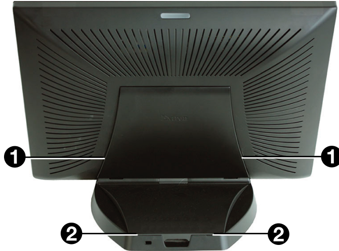
Figure 29. Remove the Rear and Base Covers
